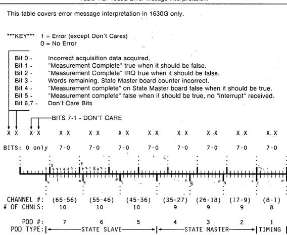
NOTE: Since the timing pod has 8 channels, the 8-bit pair of error bytes interpret directly to the timing pods' 8 channels. However, the state master pods (pods 2, 3, 4) have 9 channels, and the byte to channel interpretation is offset by one bit per pod. The State Slave pods (pods 5, 6, and 7) have 10 channels and the byte to channel interpretation is offset by two bits per pod. As in the diagram above, the bit offset must be taken into account when interpreting acquisition errors.
