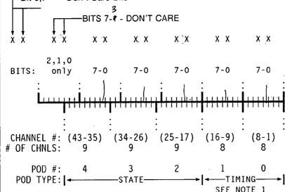
NOTE 1: In the case of timing errors, channels 8-1 actually represent the Timing Master and channels 16-9 the Timing Slave. The example above represents a 1630D. If the instrument is a 1630A, the test will show channels 16-9 as passing and channels 8-1 will represent POD 1.
