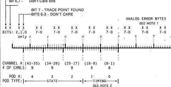
NOTE 1: Analog errors are only relevant in the 1631A/D. For 1630A/D this section of the error code will show all bits passing. For analog errors see paragraph 4-8.
